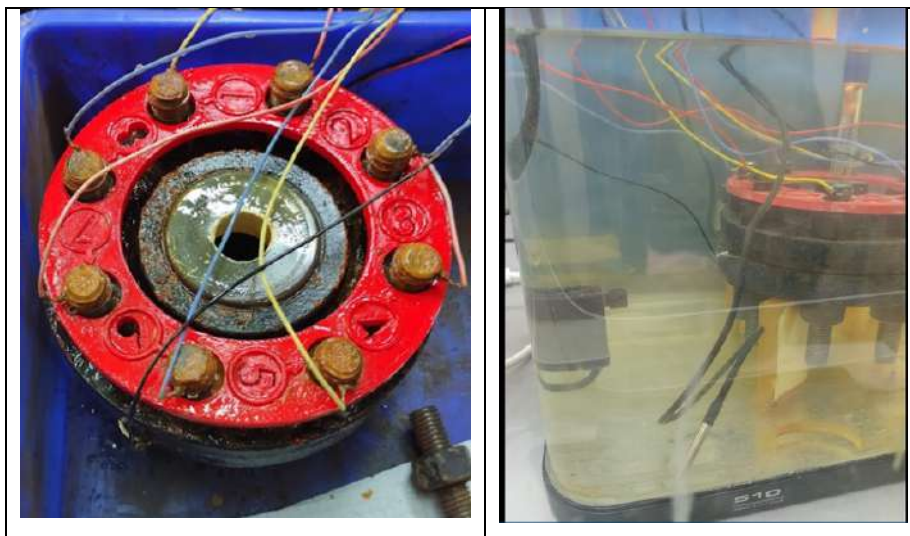
Figure 1. The flange and bolt configuration during the experiment with the ICCP system.
